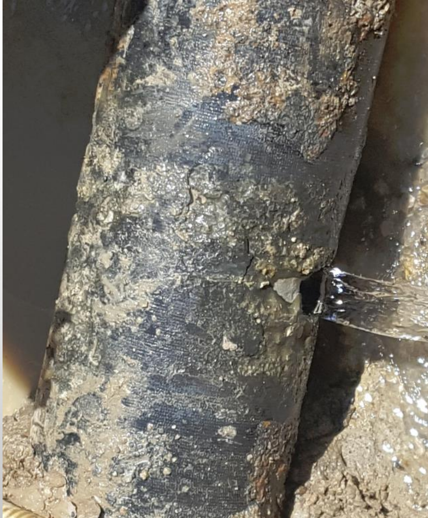
Typical Corrosive Soil Pipe Break
