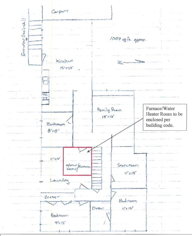
**Option 1:** This option will be required in order to bring the basement in compliance with the building code. This renovation will reduce the basement apartment to 957 square feet.
