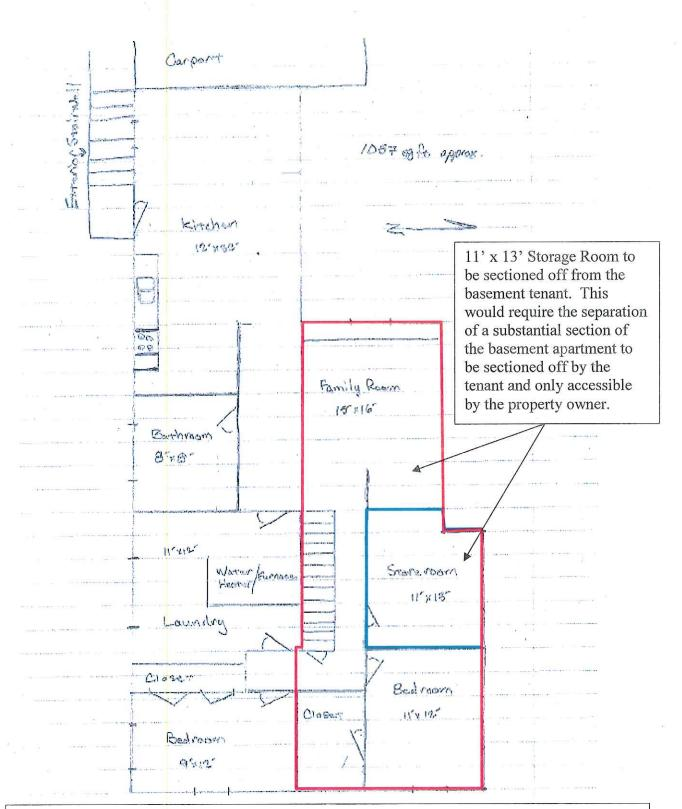
**Option 2:** This option is under the discretion of the Planning Commission. This option would bring the basement apartment under the 800 square foot requirement. This renovation would reduce the basement apartment to 658 square feet.
