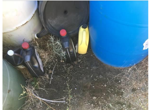
Photo #20 Staining observed by the drums of waste oil; no active leaking was observed.
