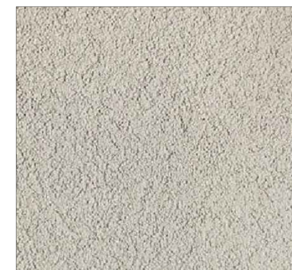
1 STUCCO MEDIUM SAND FINISH OMEGA PRODUCTS INTERNATIONAL OR APPROVED EQUAL
