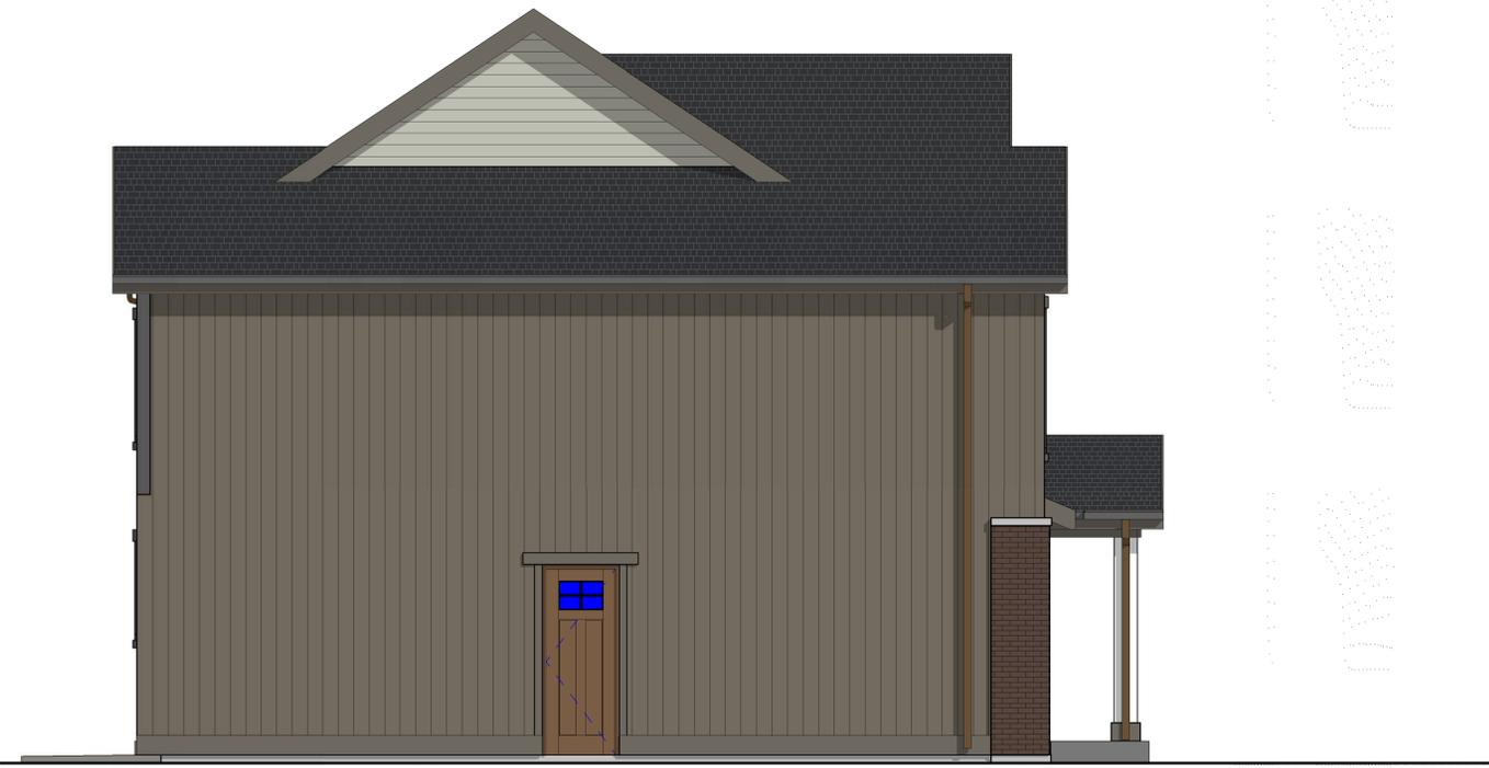
WEST DESIGN ELEVATION - BOARD & BATT
