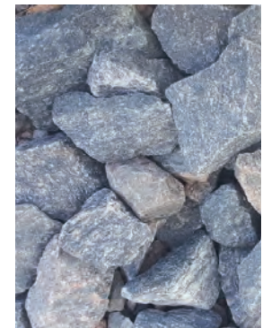
Figure 807 - 4-8 inch angular granite rubble makes a strong visual base for The Cairns's large monuments
