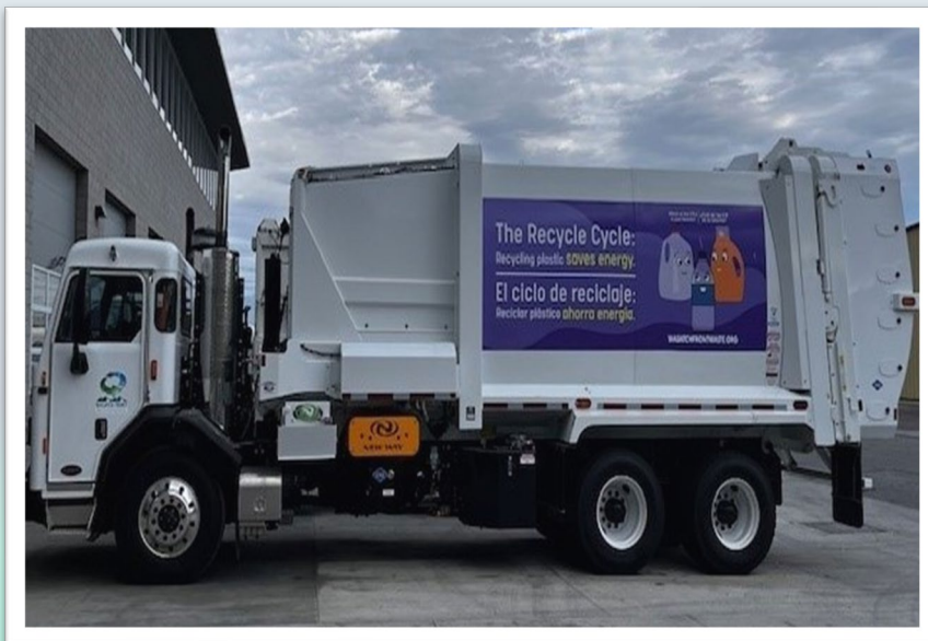
Photo of a New Side Load Truck with CNG Tanks on the Tailgate
