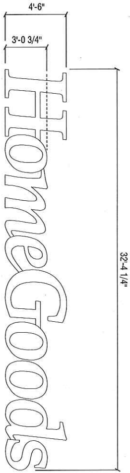
2 FRONT VIEW / SIGN B / FACE-LIGHTING CHANNEL LETTER WALL SIGN SCALE: 1/4" = 1'-0"
