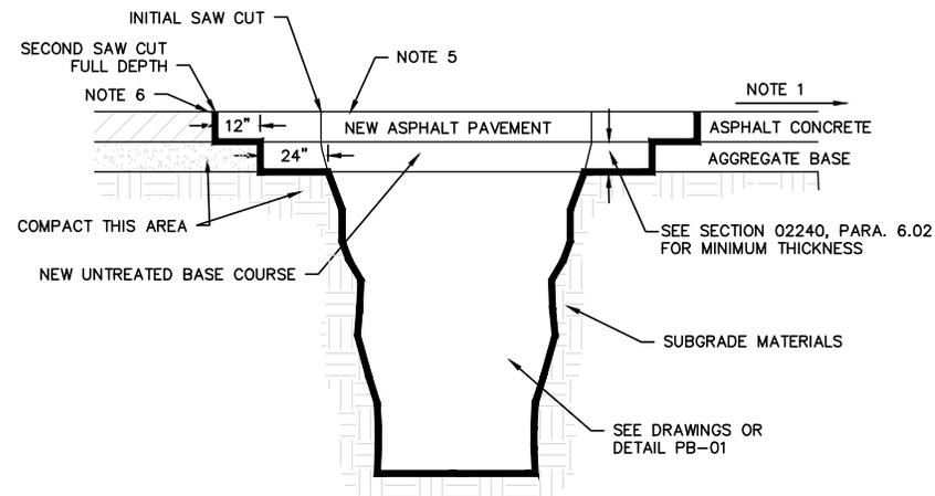
**B** DEEP EXCAVATION ASPHALT PAVEMENT
