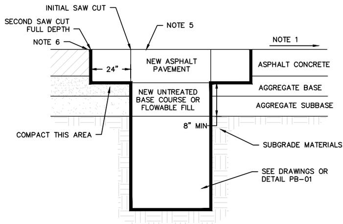
**A** SHALLOW EXCAVATION ASPHALT PAVEMENT
